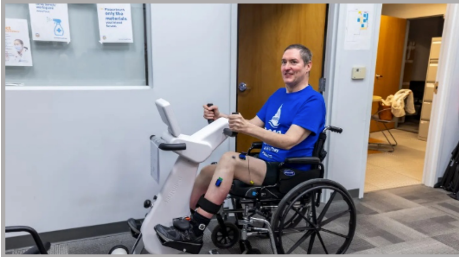
Research Participant Uses a Functional Electrical Stimulation (FES) Bite during Testing at the University of Pittsburgh
